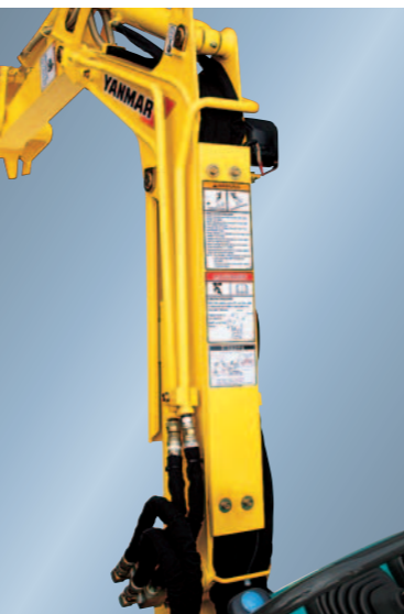
PTO PTO is piped to both right and left sides of the arm to enable the use of additional hydraulic attachments.
