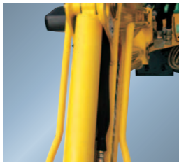
Boom cylinder and hydraulic hoses are covered for protection from accidental damage.
