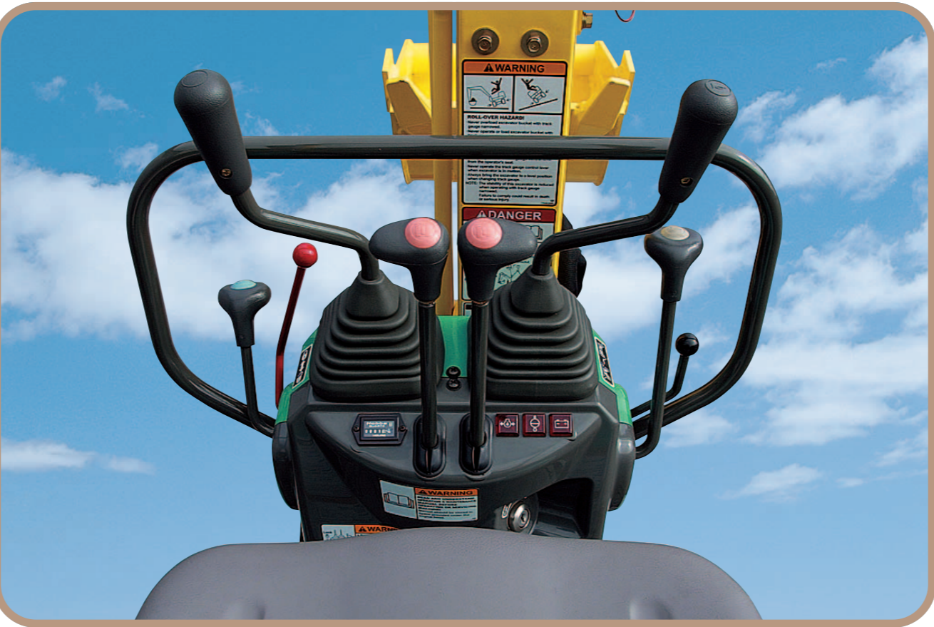
Control pattern Two-way pattern control lever is standard equipment. (ISO Excavator ↔ Optional Backhoe controls)
