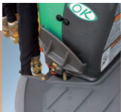
Retractable pedals PTO pedal and swing control pedal.
