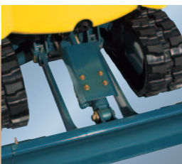
The blade hydraulic cylinder is covered by a protective shield.
