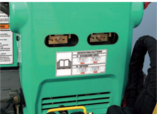
Control pattern Two-way pattern control lever is standard equipment. (ISO Excavator ↔ Optional Backhoe controls)
