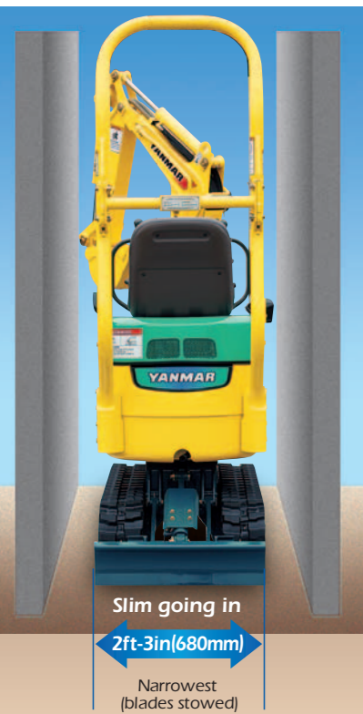
Tracks raise to 4in(100mm) for stability on slopes or steps.
