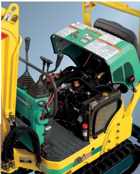
Large opening engine hood and removable side frame cover provide easy accessibility for maintenance.
