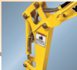
Hydraulic hoses are housed under the cylinders for protection from accidental damage.
